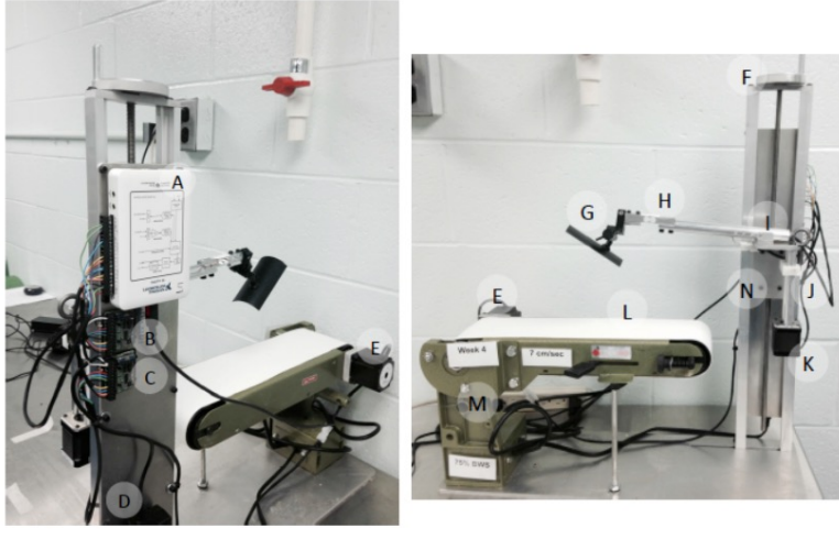
Figure 53. Custom body weight support (BWS) treadmill with components labeled. A) National Instruments myDAQ: paired with LabVIEW VI, the myDAQ issues commands to the motor controllers (B and C) and interprets the signal from the load cell amplifier (F), B) Treadmill Motor Controller: controls stepper motor used to drive the treadmill, C) Spring Tensioning Motor Controller: controls the stepper motor used to tension the spring, D) Power Supply: Supplies power to the motors, E) Treadmill Stepper Motor, F) Course Adjustment Knob: adjusts the height of the body weight support carriage, G) Animal Attachment Plate, H) Load Cell: measures the weight the animal is feeling after the spring provides assistance, I) Load Cell Amplification Circuit: amplifies the load cell signal before being processed by the my DAQ, J) Tension Spring: provides assistance to the animal when weight is supported, K) Spring Tensioning Motor: stepper motor that changes the tension of the assistance spring, L) Treadmill Belt, M) Treadmill Base, N) Body Weight Support Carriage: carriage attached to the course adjustment which moves the spring tensioning system, load cell, and variable angle specimen attachment.
